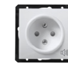
2P+PE with OP outlet single with safety shutters and overvoltage protection, (AUDIBLE ALARM) 16 A, 250 V AC, Up < 1.2 kV
