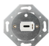
USB-C charging outlet 1 connector: USB-C charger 2,1 A, 10,5 W DSR 9C-00000-0000
