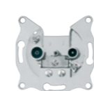
TV+R outlet through branching attenuation 9 dB for coaxial cables of diameter 4.5–8.3 mm designation on the product: ZAP 9/K
