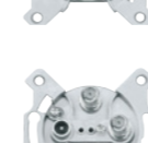
TV+SAT+SAT outlet through, attenuation 10 dB, 300 mA, 24 V DC for coaxial cables of diameter 4.5–8.3 mm designation on the product: ZAR-SAT 10/P3
